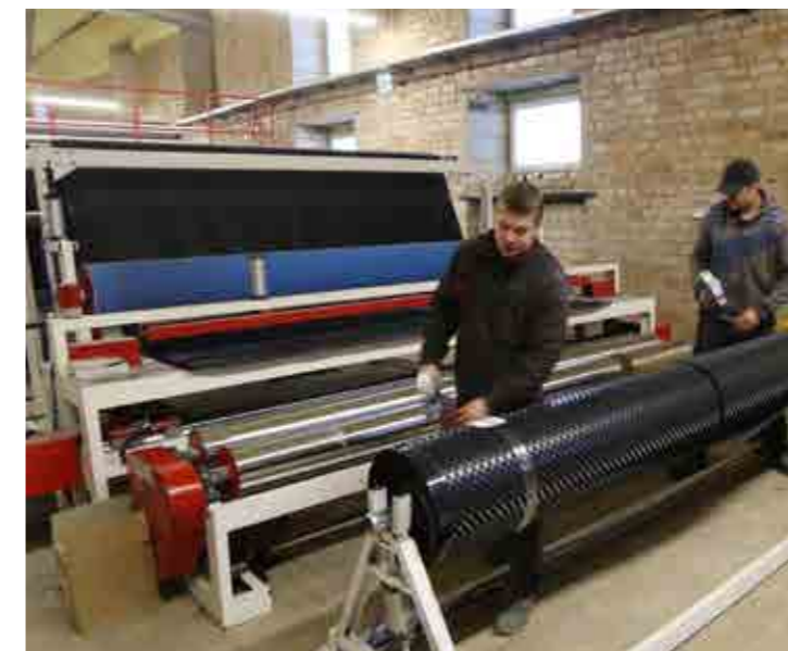
Rolled drain membrane is weighed, packed and labelled
