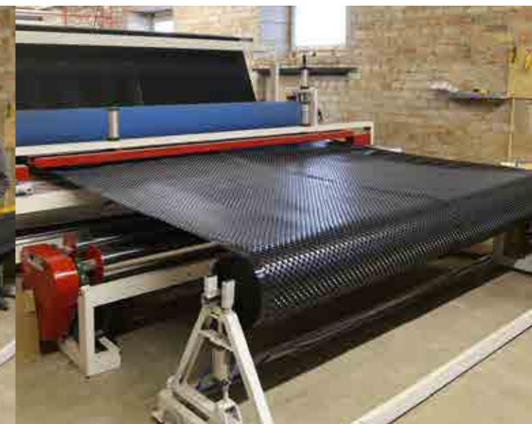
Freshly "roasted" drain membrane is being rolled
